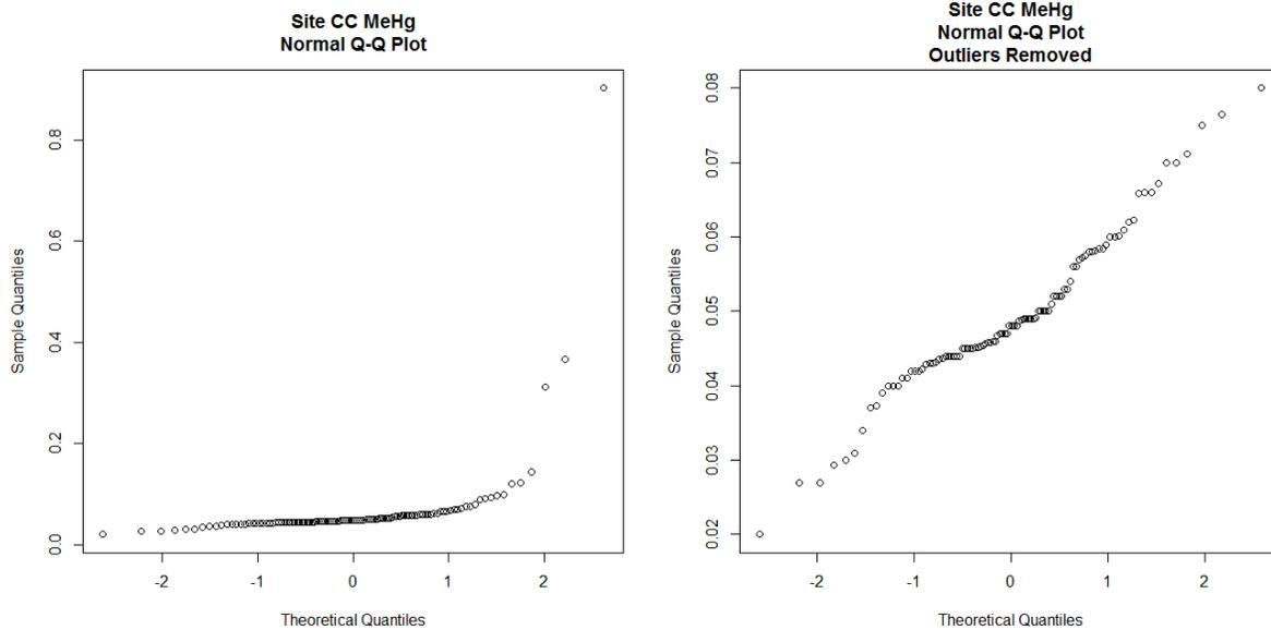
**Figure 15c.** Normal quantile-quantile plots of reported methylmercury data for site CC. All concentrations (left); non-outlier values (right).
