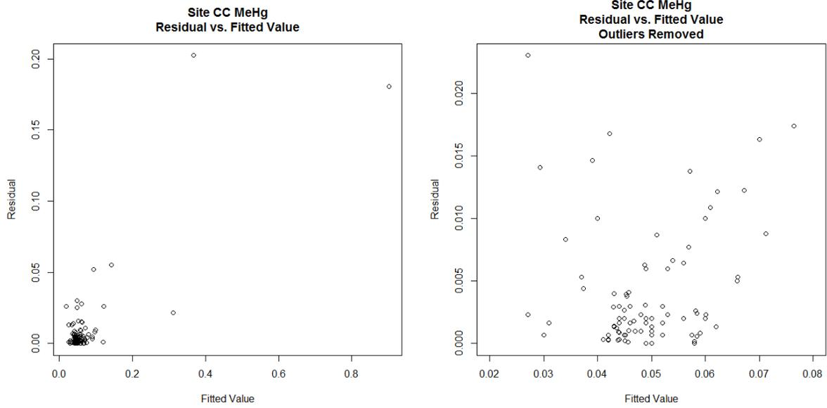
**Figure 15e.** Residual (residual = individual measurement - laboratory mean) vs. fitted value plots of reported methylmercury concentrations for site CC. All values (left); non-outlier values (right).
