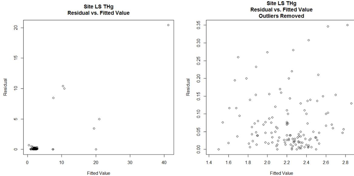
**Figure 11e.** Residual (residual = individual measurement - laboratory mean) vs. fitted value plots of reported total mercury concentrations for site LS. All values (left); non-outlier values (right).
