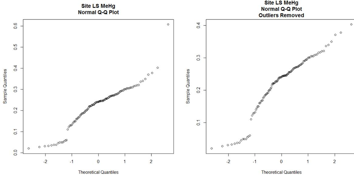
**Figure 17c.** Normal quantile-quantile plots of reported methylmercury data for site LS. All concentrations (left); non-outlier values (right).
