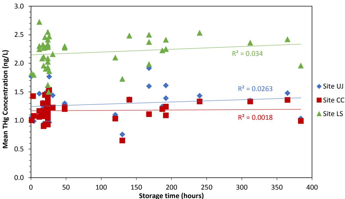
**Figure 20.** Plot of measured total mercury concentrations (lab means) vs. storage time after BrCl addition to the samples. Holding times reported as > x were substituted with x hours (the minimum time). Where a range of values was reported (e.g. 8-12 hours), the mid-point was used.
