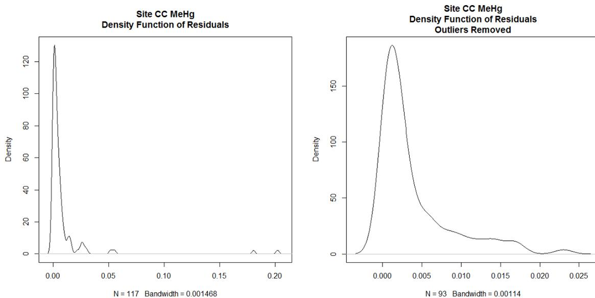
**Figure 15d.** Density functions of residuals (residual = individual measurement - laboratory mean) of methylmercury data for site CC. All values (left); non-outlier values (right).
