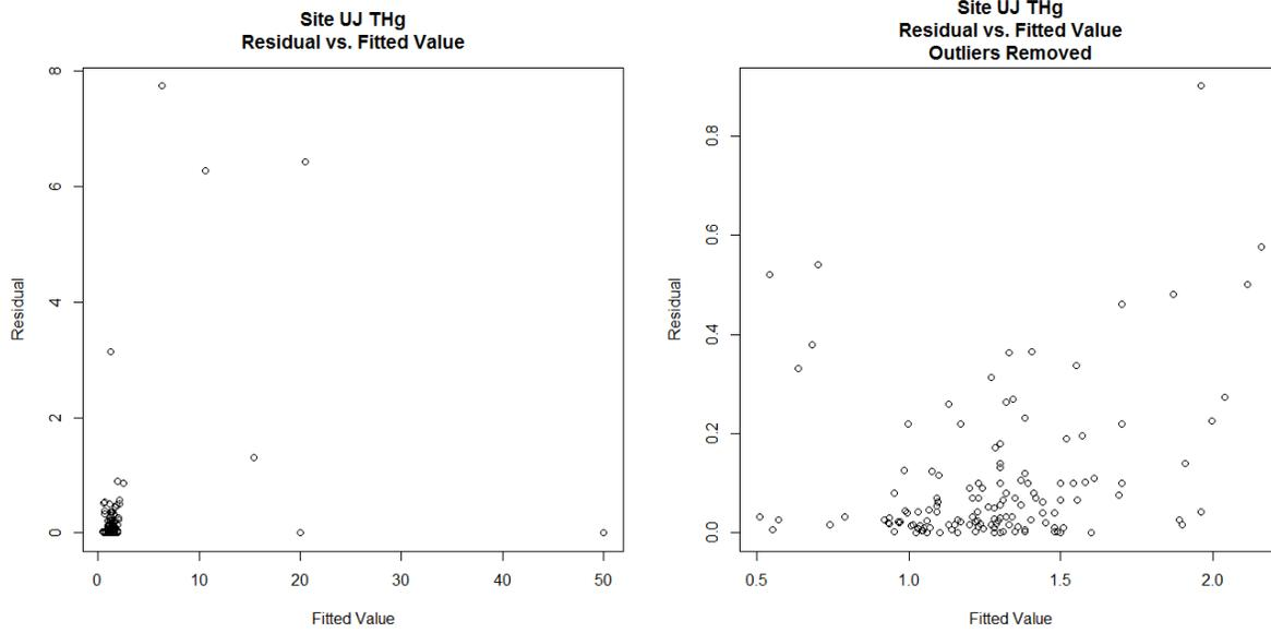
**Figure 7e.** Residual (residual = individual measurement - laboratory mean) vs. fitted value plots of reported total mercury concentrations for site UJ. All values (left); non-outlier values (right).
