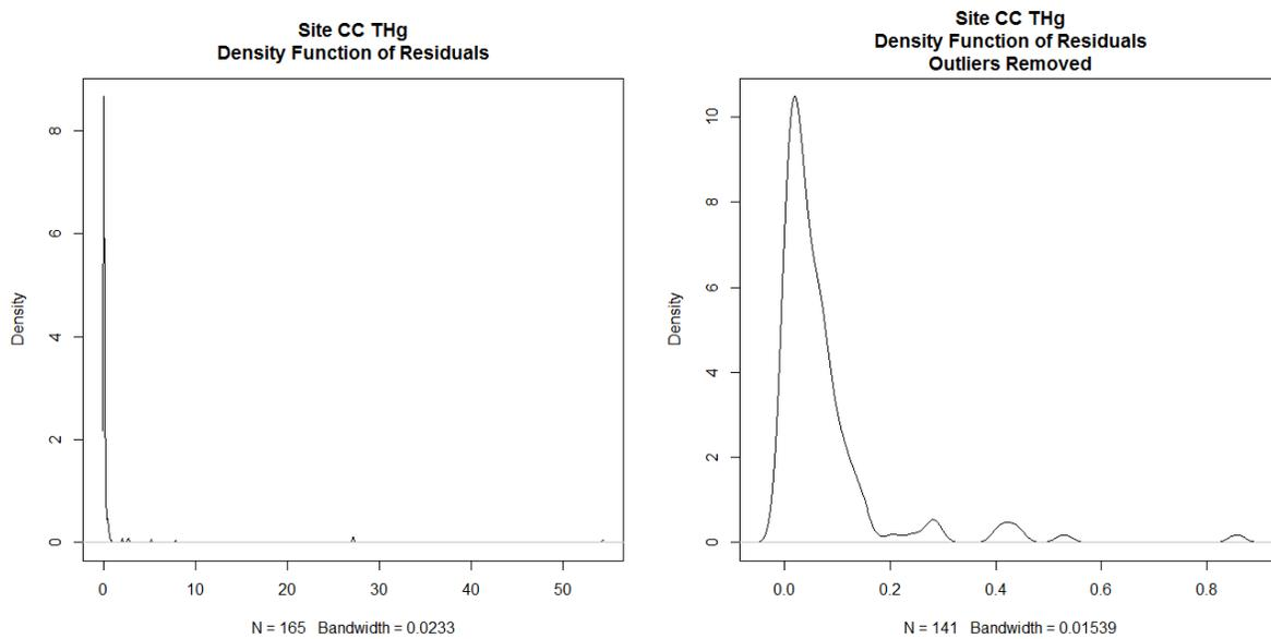
**Figure 9d.** Density functions of residuals (residual = individual measurement - laboratory mean) of total mercury data for site CC. All values (left); non-outlier values (right).
