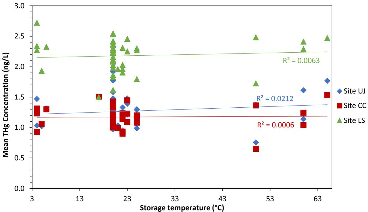
**Figure 21.** Plot of measured total mercury concentrations (lab means) vs. sample storage temperature after BrCl addition. Room temperature was assumed to be 20 °C. Where a range of temperatures was given, the midpoint was used. If samples were held at a higher temperature for several hours, followed by a lower temperature, they are plotted at the higher temperature.
