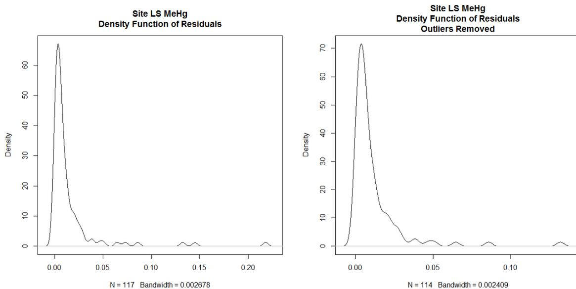
**Figure 17d.** Density functions of residuals (residual = individual measurement - laboratory mean) of methylmercury data for site LS. All values (left); non-outlier values (right).
