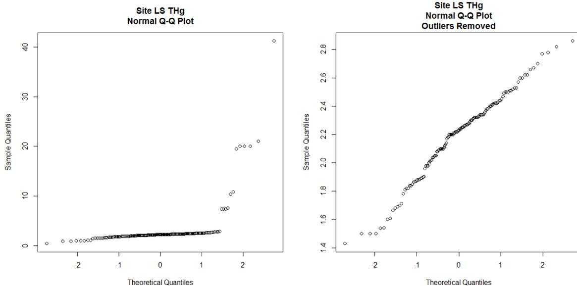
**Figure 11c.** Normal quantile-quantile plots of reported total mercury data for site LS. All concentrations (left); non-outlier values (right).
