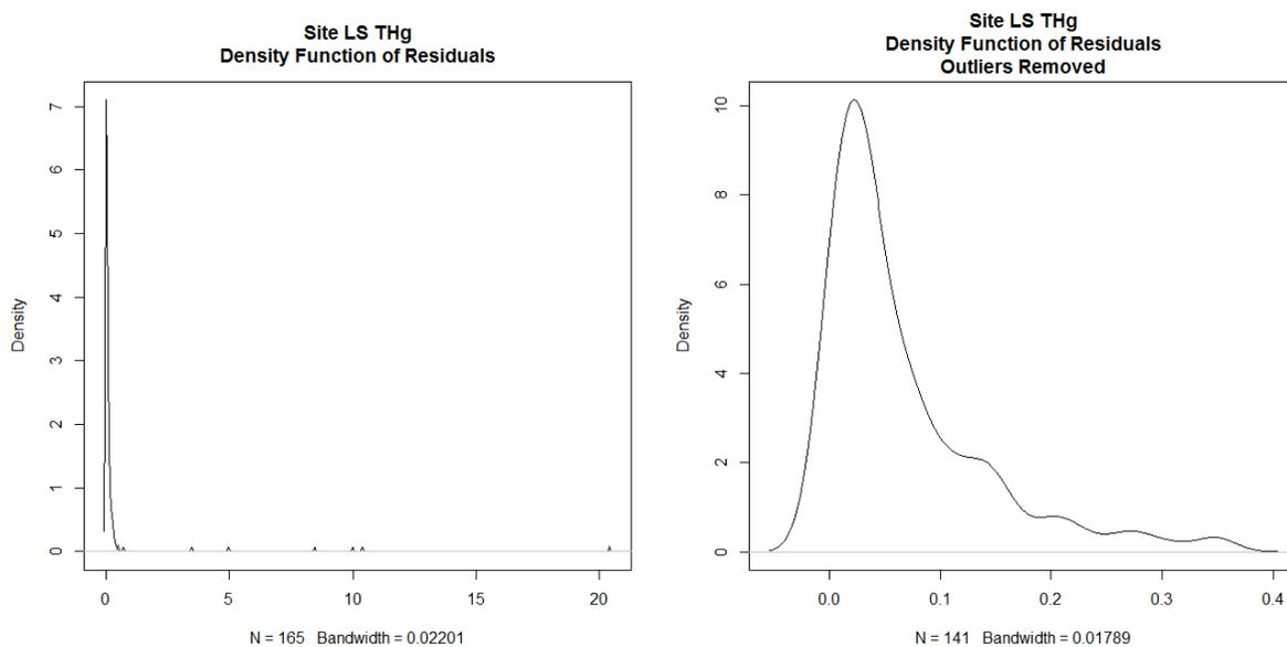
**Figure 11d.** Density functions of residuals (residual = individual measurement - laboratory mean) of total mercury data for site LS. All values (left); non-outlier values (right).
