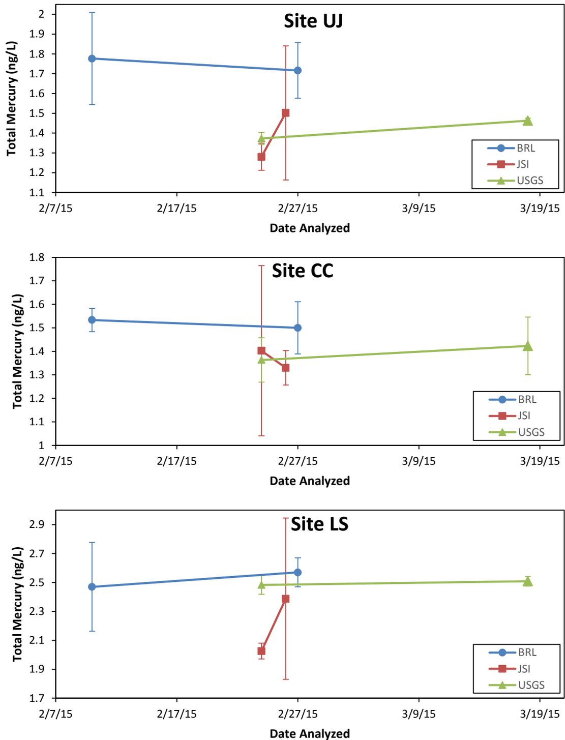
**Figure 4.** Holding time data for total mercury. Error bars are  $\pm 1$  standard deviation of replicate measurements. Where error bars are not visible, they are smaller than the chart symbol to which they pertain. Note that the vertical scales are not identical. BRL = Brooks Rand Labs; JSI = Jožef Stefan Institute; USGS = U.S. Geological Survey.
