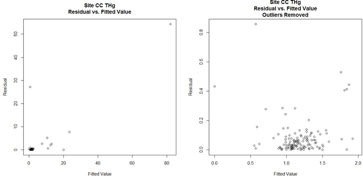
**Figure 9e.** Residual (residual = individual measurement - laboratory mean) vs. fitted value plots of reported total mercury concentrations for site CC. All values (left); non-outlier values (right).
