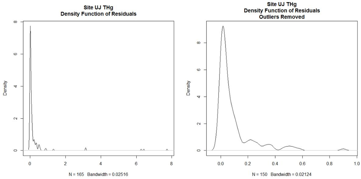
**Figure 7d.** Density functions of residuals (residual = individual measurement - laboratory mean) of total mercury data for site UJ. All values (left); non-outlier values (right).
