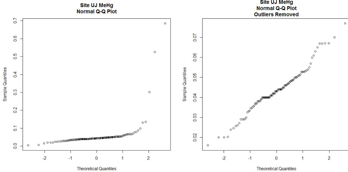
**Figure 13c.** Normal quantile-quantile plots of reported methylmercury data for site UJ. All concentrations (left); non-outlier values (right).
